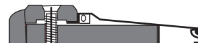
Type E = Adjustable Alum./Oak Riser Mill/Bronze Finish up To 6/0 Long Only Not Available on Mullled Units
